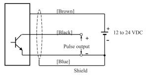
Pulse output : Open collector Max. 10 mA / 30V
