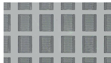
Interdigitated Capacitors (IDCs) with 2 \mu\text{m} fingers. Resist used: AZ5214E.
