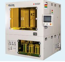
The POLOS® SPIN5000A is a stand-alone, fully automatic spin coater system. The steel housing guarantees a contamination free work area, and its high-end components ensure a repeatable, programmable spin process of up 450 x 450 mm substrates, over and over.
