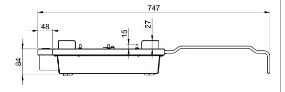
Materials: Top: Anodized Aluminium Lid Rack: Stainless Steel Frame: Antistatic POM
