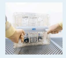
antistatic materials to protect the wafers and pod from damage or electrical shock during handling. Compliant with ISO 3 (FS209E Class 1) cleanroom standards, it ensures safe operation in sensitive semiconductor environments.
