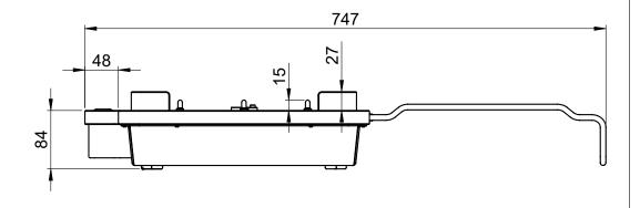
Materials: Top: Anodized Aluminium Lid Rack: Stainless Steel Frame: Antistatic POM
