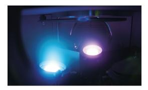
lon source can be used to clean the substrate and accelerate the sputtering speed of the coating material, and the ion beam helps deposit and compact the deposited films during the material deposition process.
