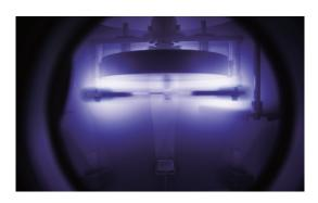
This sputter system can independently apply bias voltage on its stage part to clean and increase the adhesion of materials.
